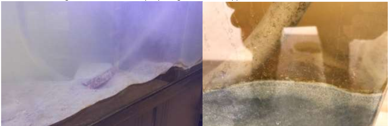
Figure 9: Images shows testing tank after (5) days of testing and color changing in sediment top layer (Right image)
