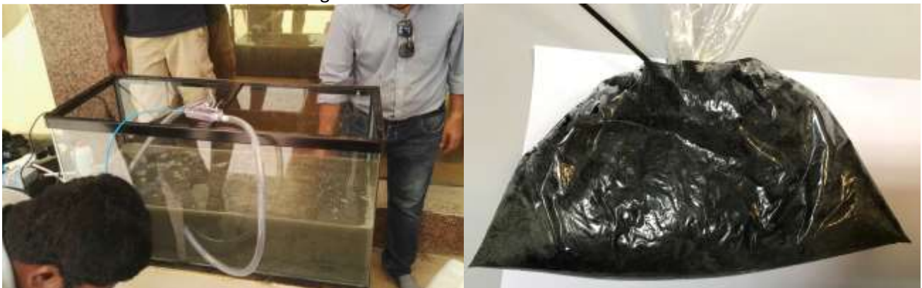
Figure 7: (Left) image shows seawater color after mixing with sediment, (Right) image shows sediment samples showing contaminated sludge content
